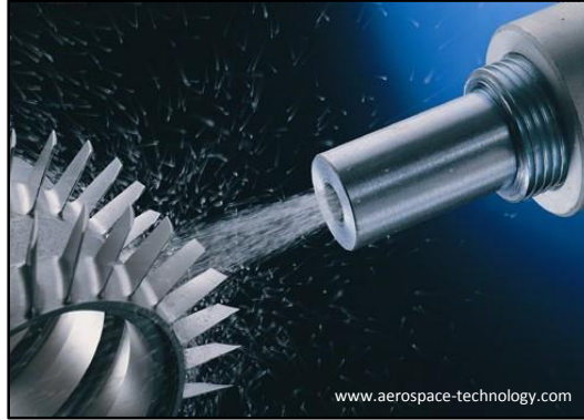
Figure 2-1 Shot peening (SP).
